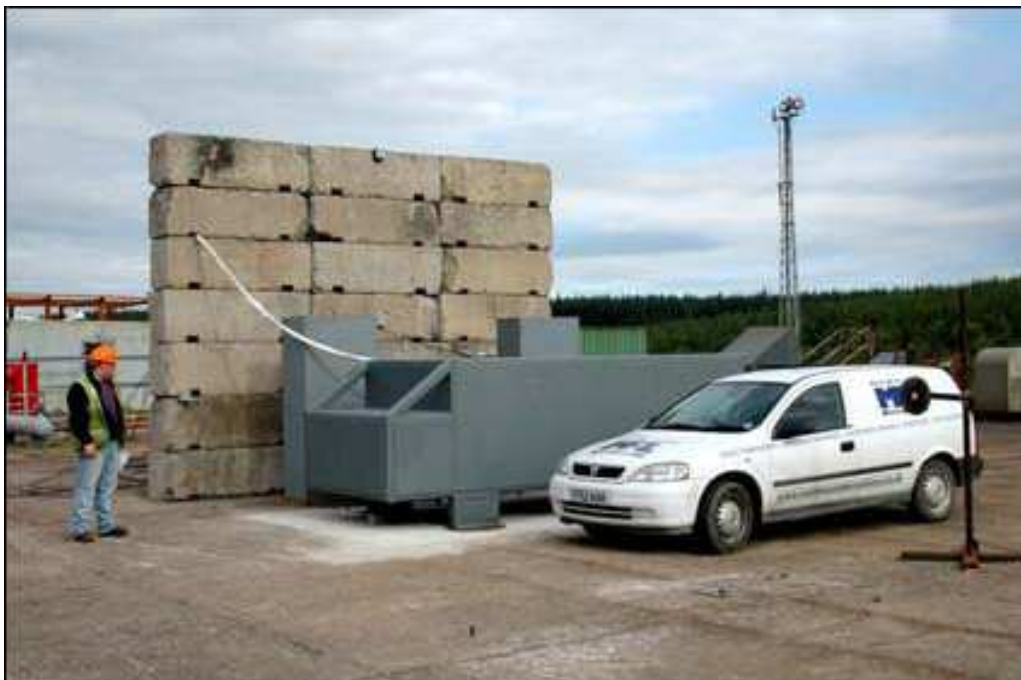
Figure 2 View of refuelling station model used in jet release experiments. Comparison with real car
