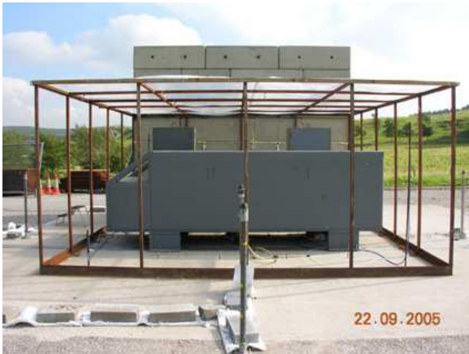
Figure 1 View of refuelling station model used in premixed experiments. Plastic film covering the frame is not shown
