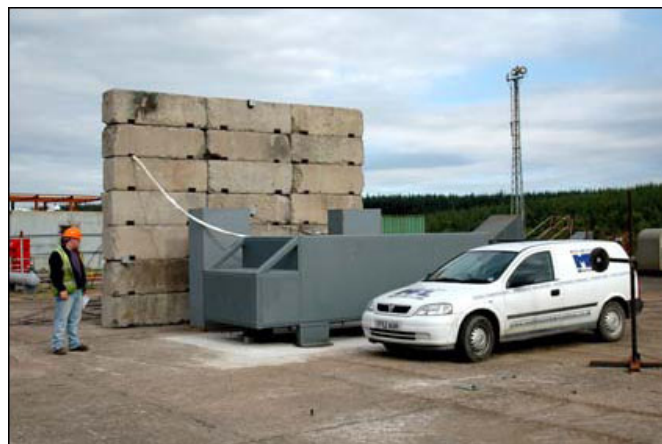
Figure 2: The refuelling station model used in the jet release experiments (comparison with real car) (Shirvill et al., 2007).
